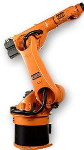
Robot control software can undertake flexible programming process for 3-dimensional welding , and can be freely combined with the peripheral devices. Control system function can be set with different packages to meet the individual needs of different customers.
