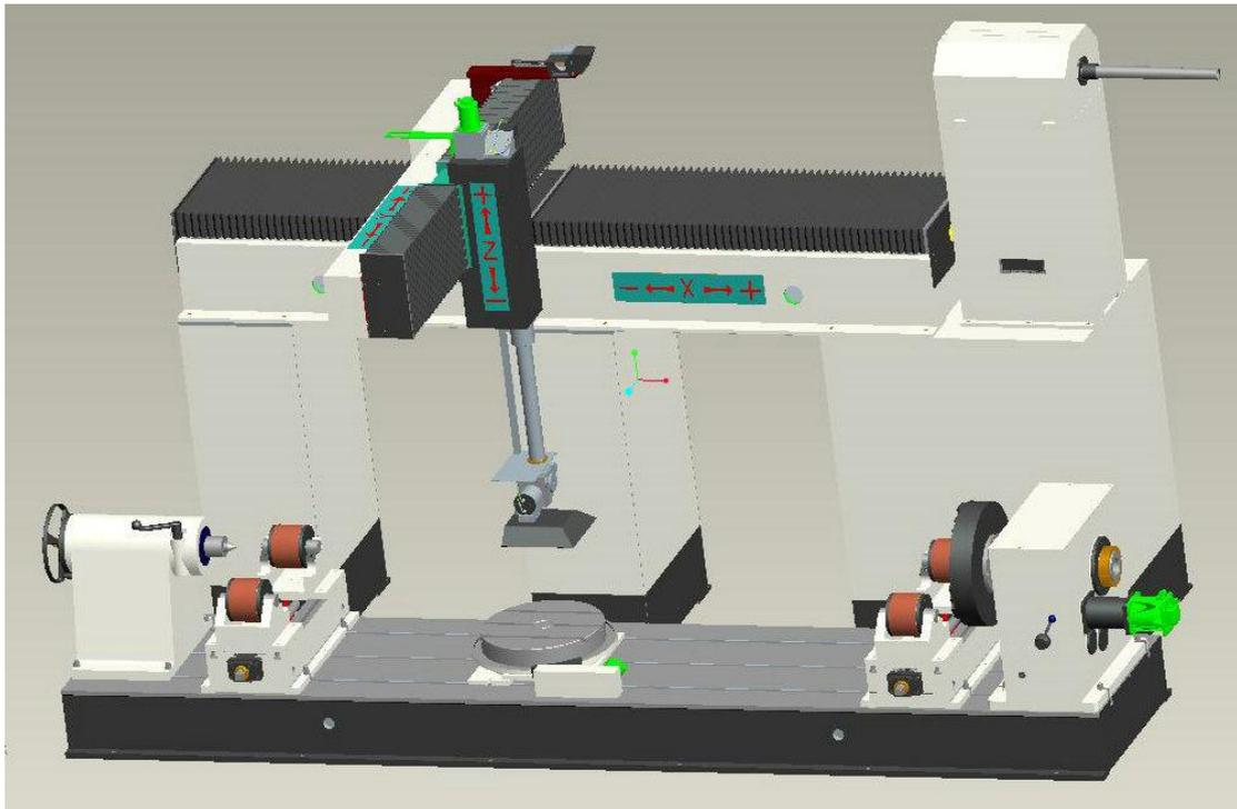
Adopting **bracket -movement style** flight path movement form,with X Y Z 3 axis linear motion function and swing function; machine tool equipped one horizontal rotary worktable(C axis);X,Y.Z and C axis form a four axis five linkage processing system.
